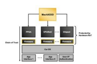
The Lattice MachXO3D FPGA for secure control in automotive applications establishes a hardware Root-of-Trust to confirm that the device, and other devices that boot after the FPGA, are running authorized firmware. (Graphic: Business Wire)
