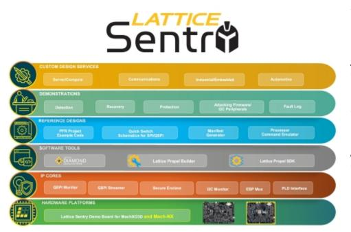
The Lattice Sentry solutions stack helps developers create cyber resilient system control applications compliant with NIST guidelines for platform firmware security (NIST SP-800-193). It consists of a complete reference platform, fully validated IP building blocks, easy-to-use FPGA design tools, reference designs, and a network of custom design services. (Photo: Business Wire)
